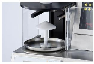
A conical funnel, which can be equipped with different pouring nozzles, takes the sample to be tested. A built-in analytical Sartorius balance cell takes the product collecting dish. The PTG-ER electrical stirrer may be used for powders, which do not flow well. Most pharmaceutical material contains such a high amount of fine particles that it will not start to flow without assistance.
