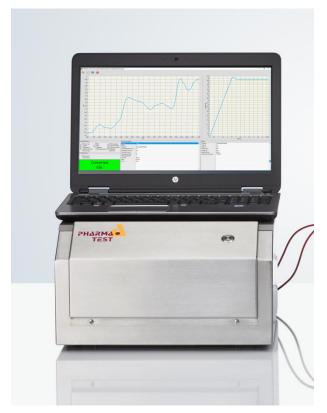
The TIDAS L NIR is a diode array spectrometer. This technology is much faster compared to common scanning spectrophotometers. Instead of of the sequential scanning technique, the full spectrum is immediately detected and multiple wavelenghts may be examined at the same time. This way even fast spectral changes can be detected by the diode array spectrometer. The TIDAS L NIR provides excellent signal to noise ratio to detect even weak signals.
