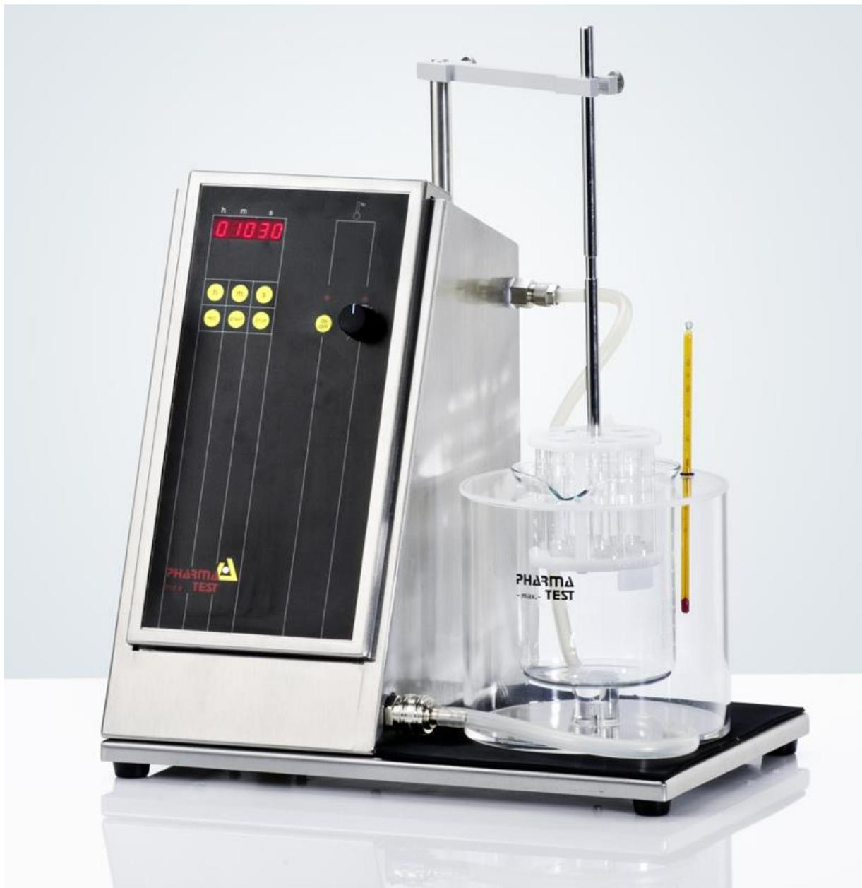
The PTZ-S is used for the manual testing of disintegration times of tablets, capsules and other solid dosage forms. The single basket PTZ-S version offers the following features:
