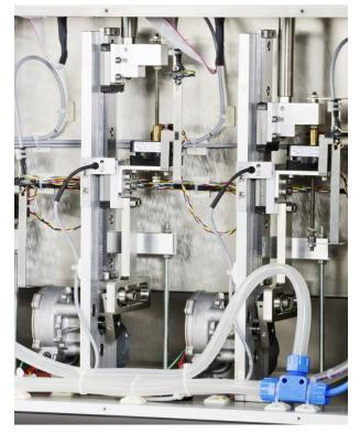
For easy cleaning and maintenance, the Plexiglas water bath can be easily removed. Fast Tube Couplings connect the tubing to the heating system. The digital controlled stroke mechanism is automatically adjusted to provide the USP / EP specified 30 strokes a minute to each station.
